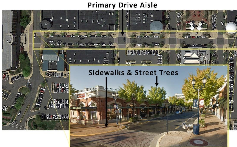
Figure 5-6: Design of Primary Drive Aisle
